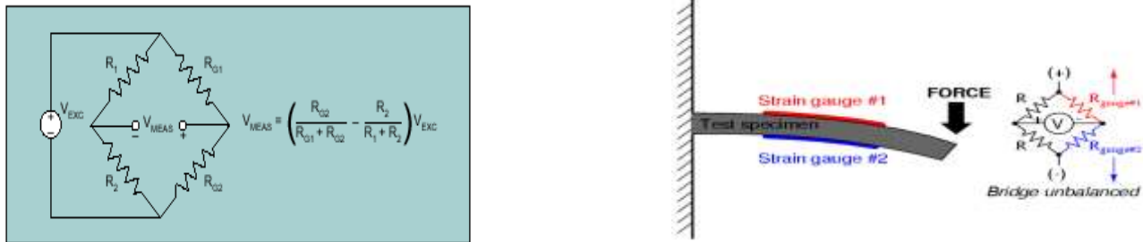
Figure 4.2: Half-Bridge Strain Gauge Configuration
